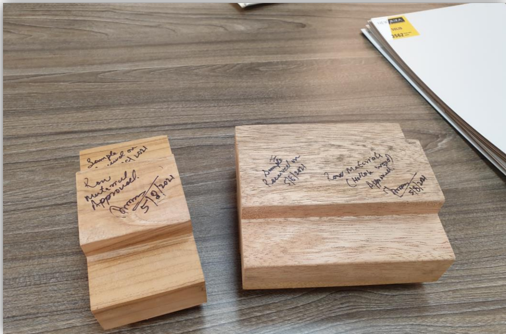
HOLLOCK WOOD & TEAK WOOD SEGREGATION FOR CLIENT'S
